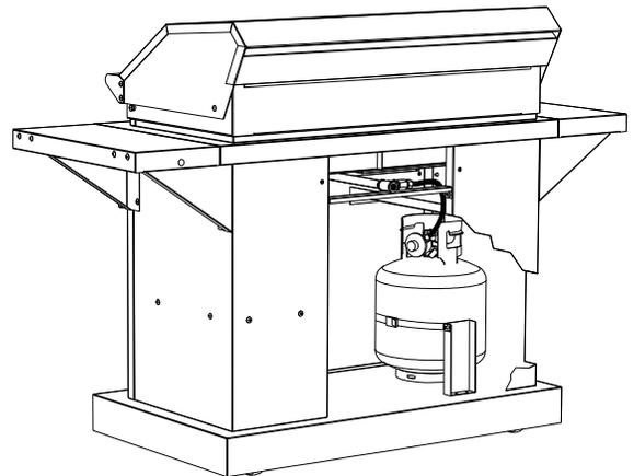
**Important:** The regulator hose assembly is connected at the factory before shipping. If the regulator ever needs to be replaced, the work must be done by a qualified technician.
