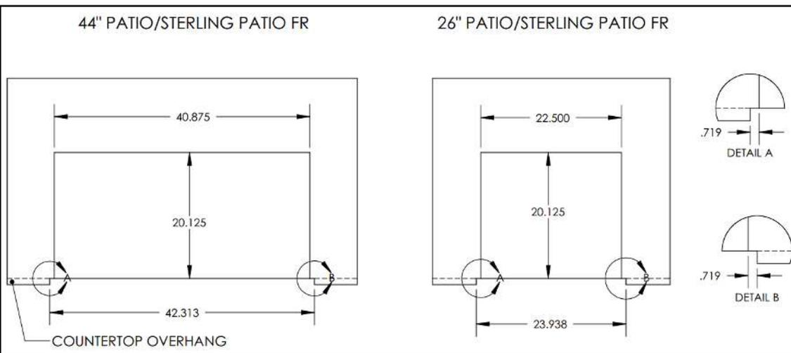
Countertop Overhang Notch: The countertop overhang must be horizontally notched out .719" on either side of the cut out opening for the grill to accommodate the control panel (See Detail A&B).
