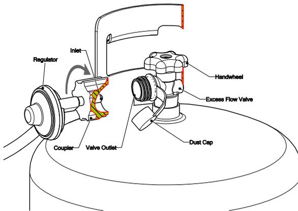
**Warning:** Do not use any other regulator/hose assembly other than the one supplied with your grill. If the regulator/hose assembly needs replacing, use only TEC specified replacement parts.
